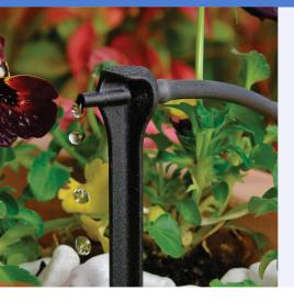
A landscape and nursery dripper incorporating an anchoring spike that delivers precise amounts of water direct to the plant root zone. Asta<sup>®</sup> pressure compensating (PC) spike dripper has a sealed turbulent flow path and diaphragm to maintain uniform discharge rates over a wide range of pressures.
