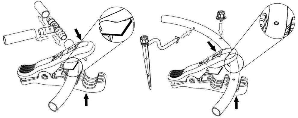
Cuts low density poly pipe and vinyl tubing up to 22 mm OD.
