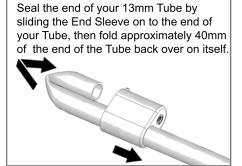
Slide the End Sleeve back over the bent end of the 13mm Tube to hold it in the folded postition. If you need to flush dirt out of your lines, you can slide the End Sleeve off again to clean the Tube.
