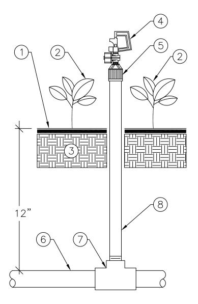
NOTE: SET ZONE PRESSURE TO 30 PSI. ADJUST VARI—ROTOR SPRAY DIAMETER AS NEEDED.
